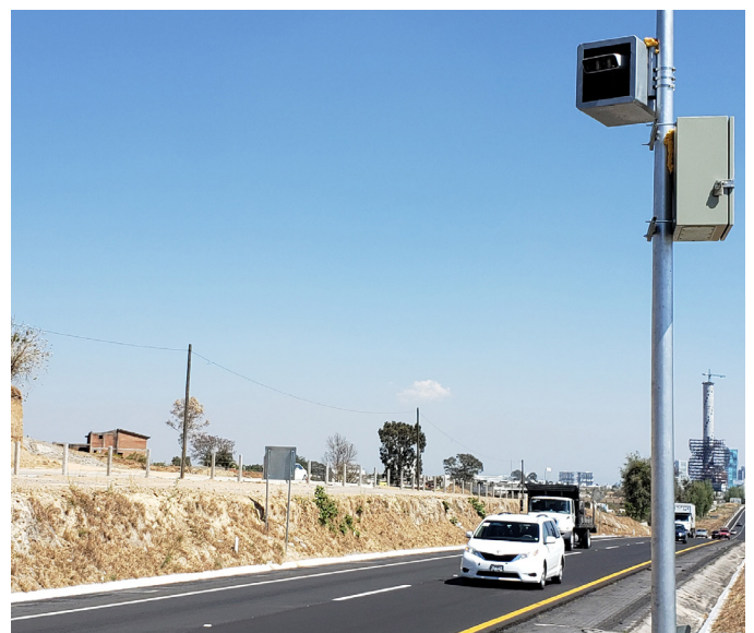
A TrafficCam 3D monitors speed near a busy roadway in Mexico City
