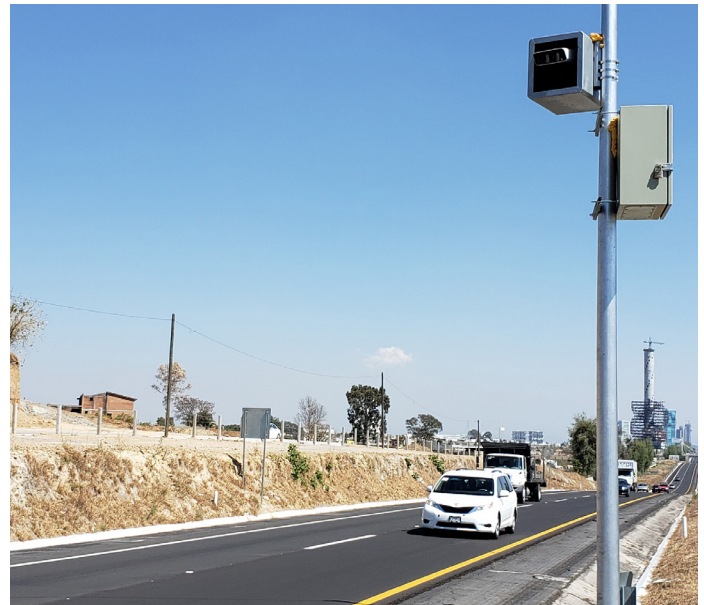
A TrafficCam 3D monitors speed near a busy roadway in Mexico City
